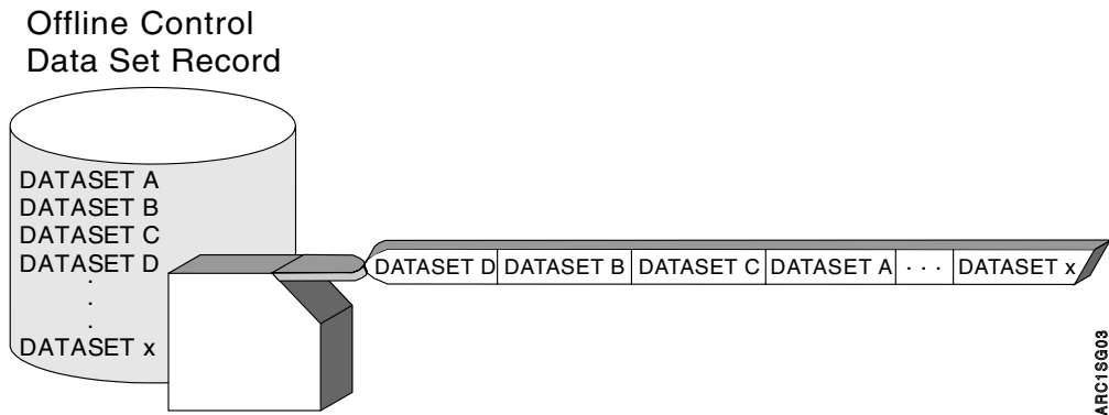
Figure 78. Creation of Tape Data Set Copies. DFSMSHsm makes an entry in the offline control data set record for each data set stored on a migration or backup tape.
